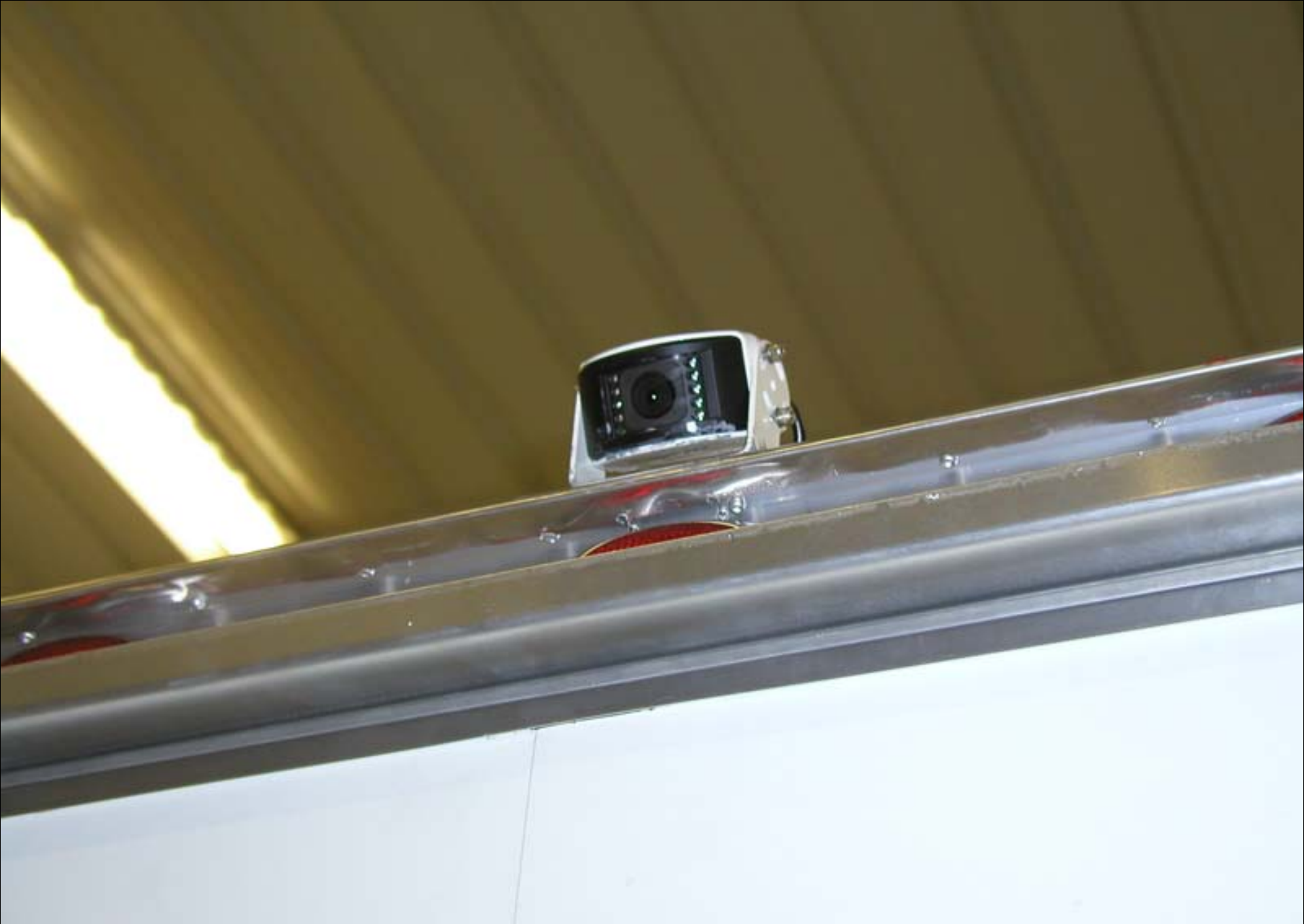
REMOTE CAMERA MOUNTED AT EXTERIOR REAR ABOVE RAMP DOOR
